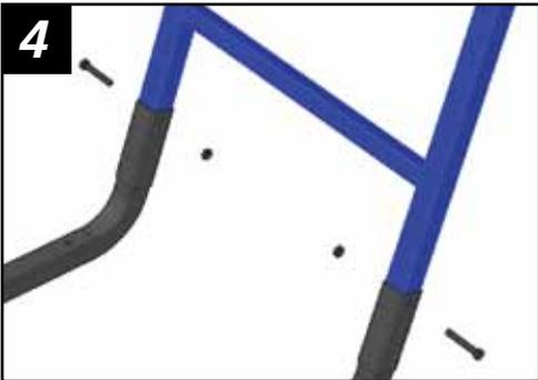
**2 1/2" BOLTS, LOCK NUTS - WRENCH TIGHTEN STEP 7**
