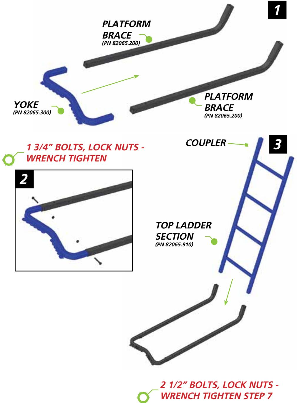
**1 3/4" BOLTS, LOCK NUTS - WRENCH TIGHTEN STEP 7**
